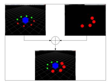
Note that we could also enable blending in the fragment shader. Assuming that the two images to be blended are bound to their texture units and their shader samplers are texture1 and texture2, the additive blending shader code will be like this:
