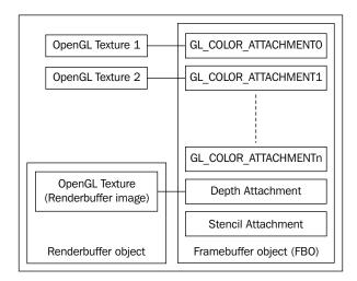
If depth testing is required, a render buffer is also generated and bound by calling glGenRenderbuffers followed by the glBindRenderbuffer function. For render buffers, the depth buffer's data type and its dimensions have to be specified. After all these steps, the render buffer is attached to the frame buffer by calling the glFramebufferRenderbuffer function.
