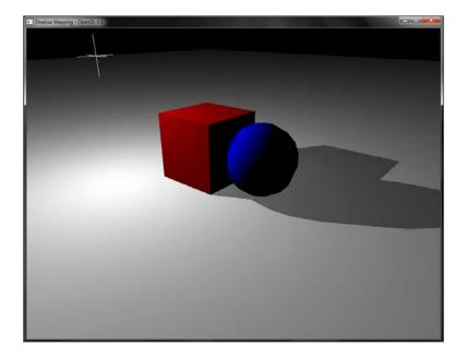
This recipe detailed the shadow mapping technique for a single light source. With each additional light source, the processing, as well as storage requirements, increase.
