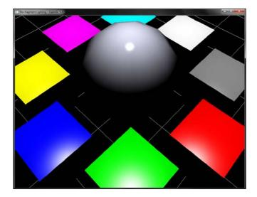
Note how the per-fragment lighting gives a smoother result compared to the per-vertex lighting. In addition, the specular component is clearly visible.
