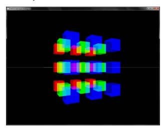
Pressing the Space bar disables front-to-back peeling so that we can see the normal alpha blending without back-to-front sorting which gives the following output. Note that we do not see the yellow blended color where the green and red boxes overlap.
