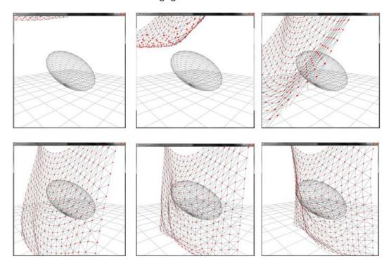
Although we have touched upon basic collision primitives, like spheres, oriented ellipsoids, and plane, more complex primitives can be implemented with the combination of these basic primitives. In addition, polygonal primitives can also be implemented. We leave that as an exercise for the reader.
