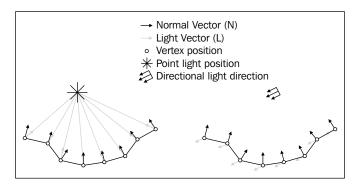
The figure compares directional and point light sources. For a point light source (left-hand side image), the light vector at each vertex is variable, depending on the relative positioning of the vertex with respect to the point light source. For directional light source (right-hand side image), all of the light vectors at vertices are the same and they all point in the direction of the directional light source.
