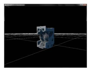
Note that we cannot see the black halo around the volume dataset as was evident in earlier recipes. The reason for this is the if condition used in the fragment shader. We only perform these calculations if the current density value is greater than 0.1. This essentially removed air and other low intensity artifacts, producing a much better result.
