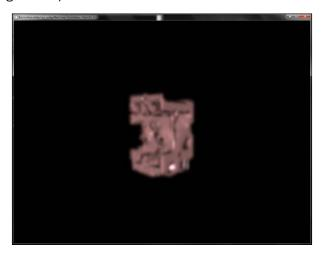
This recipe gave us an overview on the splatting algorithm. Our brute force approach in this recipe was to iterate through all of the voxels. For large datasets, we have to employ an acceleration structure, like an octree, to quickly identify voxels with densities and cull unnecessary voxels.
