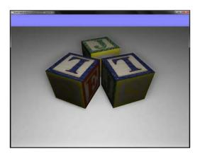
Pressing the Space bar disables SSAO to produce the following output. As can be seen, ambient occlusion helps in giving shaded cues that approximate how near or far objects are. We can also change the sampling radius by using the + and - keys.
