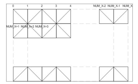
In order to alternate the triangle directions and maintain their winding order, we take two different combinations, one for an even iteration and second for an odd iteration. This can be achieved using the following code:
