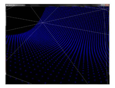
When in the camera 2 view (see the following figure), we can click-and-drag the left mouse button to rotate camera 1. This allows us to see the updated viewing frustum and the visible points. In the camera 2 view, visible points in the camera 1 view frustum are rendered in magenta color, the viewing frustum planes are in red color, and the invisible points (in camera 1 viewing frustum) are in blue color.
