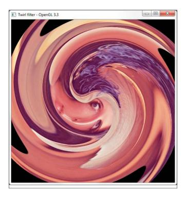
Since the texture clamping mode was set to <code>GL\_CLAMP\_TO\_BORDER</code>, the out of image pixels get the black color. In this recipe, we applied the twirl effect to the whole image. As an exercise, we invite the reader to limit the twirl to a specific zone within the image; for example, within a radius of, say, 150 pixels from the center of image. Hint: You can constrain the radius using the given pixel distance.
