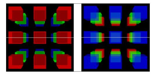
Depth peeling (also called front-to-back peeling) is one technique that helps in this process. In this technique, the scene is rendered in slices in such a way that slices are rendered one after another from front to back until the whole object is processed, as shown in the following figure, which is a 2D side view of the same scene as in the previous figure.
