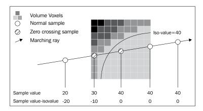
Next, we use the Phong illumination model to render the shaded isosurface and break out from the ray marching loop. Note that the method shown here renders the nearest isosurface. If we want to render all the surfaces with the given isovalue, we should remove this break statement.
