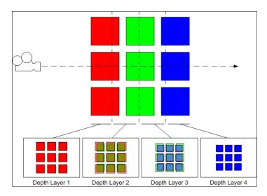
The number of layers to use for peeling is dependent on the depth complexity of the scene. This recipe will show how to implement this technique in modern OpenGL.
